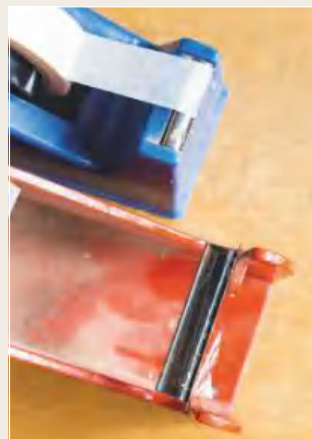
Darren's incredibly clever yet simple tape dispenser for working with veneers
